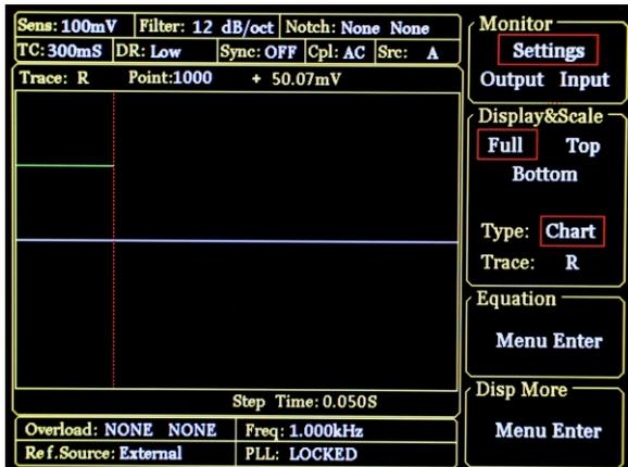
In addition, OE1022 can also use polar coordinates to display the in-phase component and quadrature component of the input signal. All of these display modes can be easily adjusted by manual or automatic operations.
